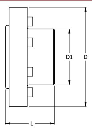
D = 440 D1 = 265 L = 180 Max bore = 160 Torque (N m) = 13500
